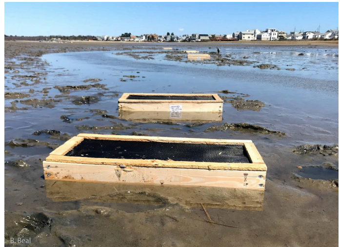
A 1 foot x 2 feet x 3 inch deep soft-shell clam recruitment box. The empty boxes were anchored to the mudflat surface during the last two weeks of May and remained in place until the first two weeks of November.
